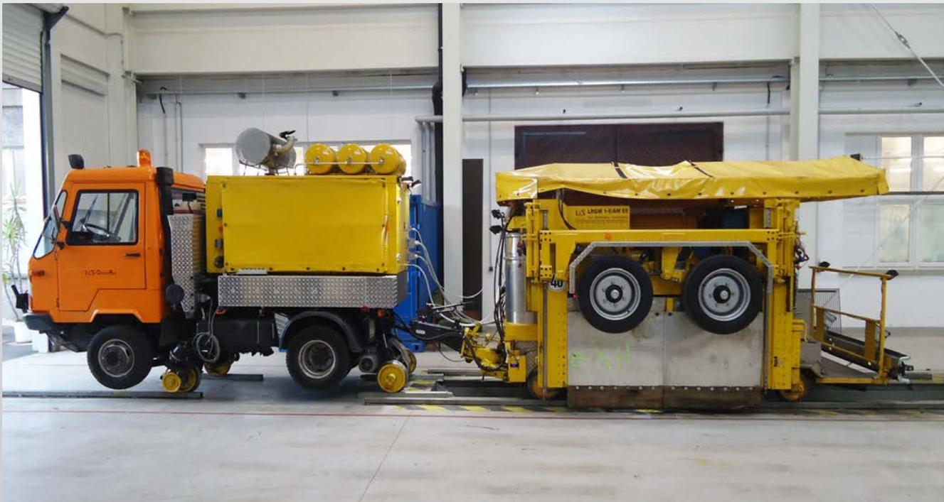
The RRG 1-6/ AM 65 is a road-rail going grinding machine for the machining of the rail head of tracks and turnouts. It composes except the grinding wagon also a generator so that no power cables has to be installed along the working site. The grinder can travel flexibly to the position for rail-in und easily rail in and out by road-rail technology.
